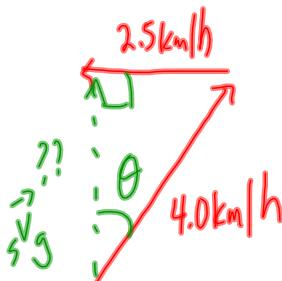
$$\begin{aligned}c^2 &= a^2 + b^2 \\4.0^2 &= 2.5^2 + b^2 \\b^2 &= 4.0^2 - 2.5^2\end{aligned}$$
